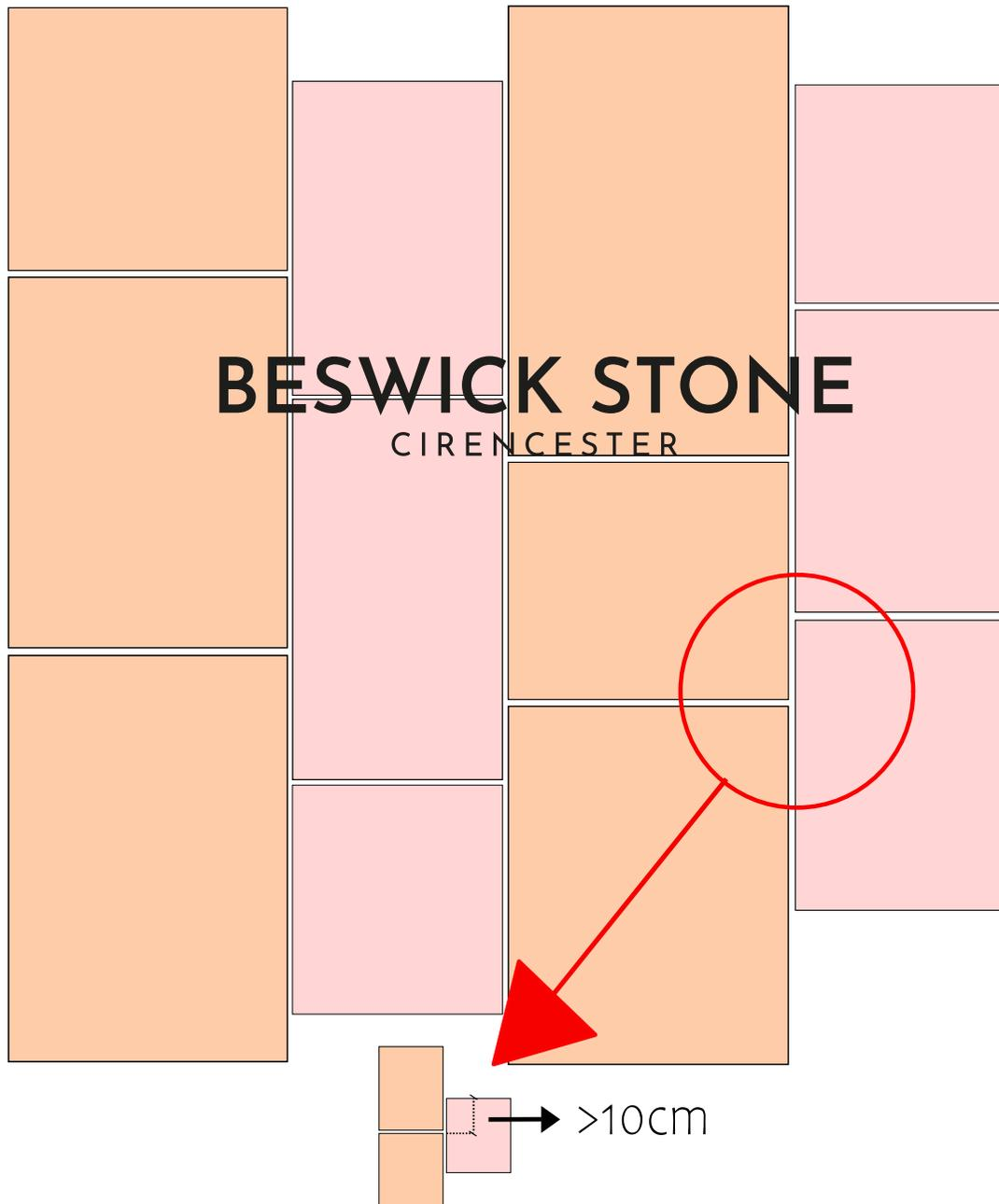
**Laying tip: there is NO pattern to follow, simply lay the stones in straight rows, aim for no less than 10cm between the short side grout joint from row to row.**
